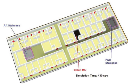
Figure 3. Overview of the deck at time 430 s. Fire case scenario—ignition at cabin M5.
