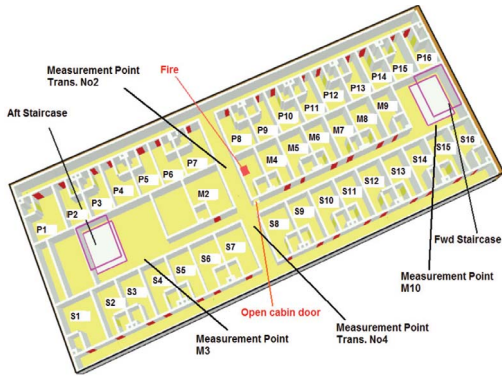
Figure 1. Deck overview showing the cabins and the location of measurement devices.
